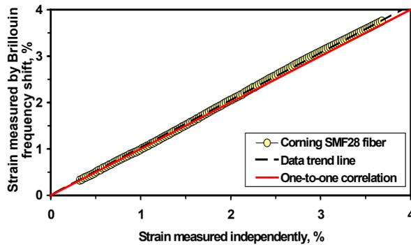
Figure 3. Calibration verification of Brillouin based strain with independently measured strains
