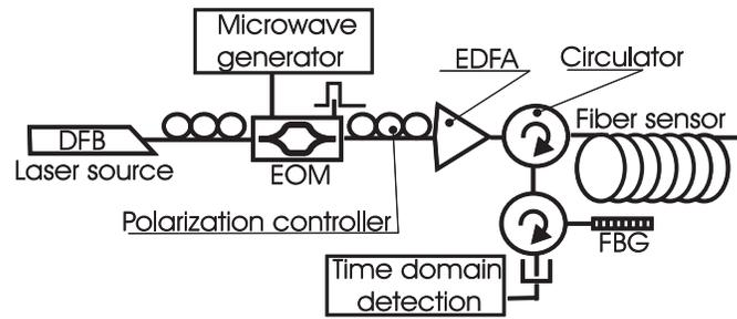
Figure 1. Lehigh's frequency modulated Brillouin photonics assembly
