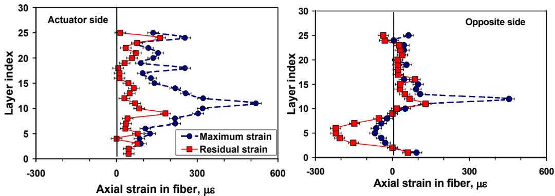
Figure 6. Strain measurement in fiber layers during and after the load
