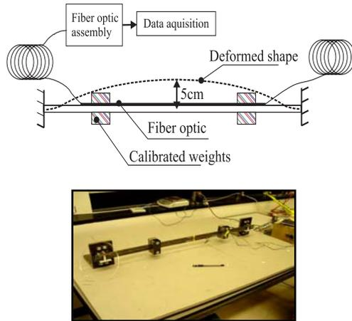
Figure 7. Oscillation test set-up
