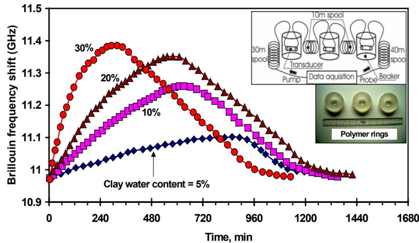
Figure 4. Brillouin signal shift as a function of swelling/shrinkage time and clay water content (inset – sketch of experimental set up and picture of polymer rings)
