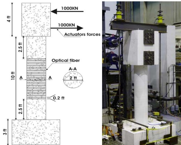
Figure 5. Large-scale test column with optical fiber layout (Lehigh George E. Brown, Jr. NEES laboratory)
