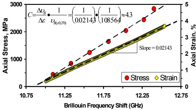
Figure 2. Brillouin frequency with independently measured stress & strain to *Corning SMF28* fiber
