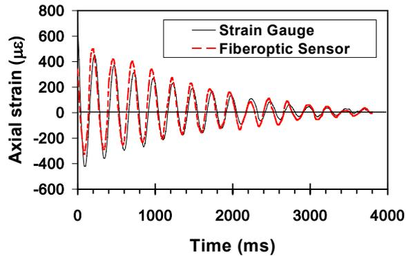
Figure 8. Damped oscillation measurements using the fiber optic sensor and strain gauge
